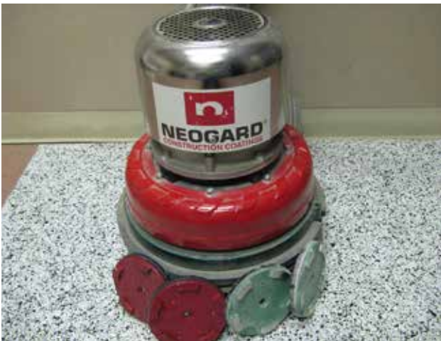
Floor grinder w/diamond grinding discs
