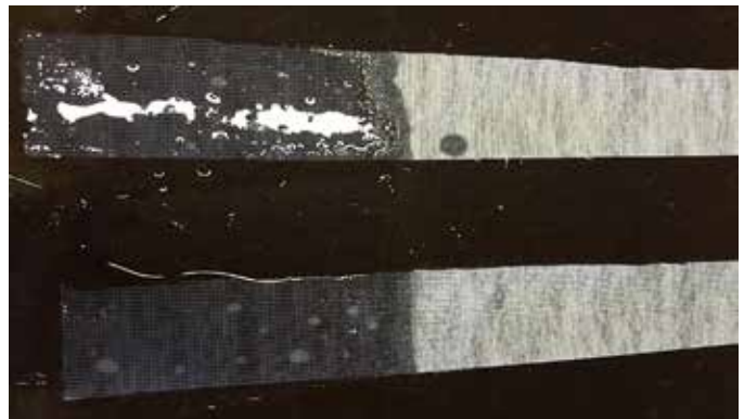
Fabric strips worked into wet coating
